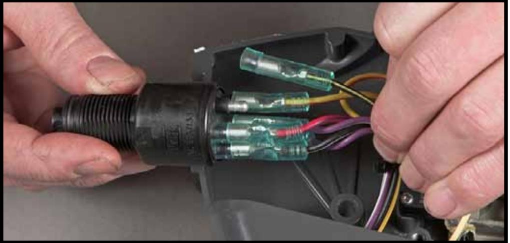
(You might need to pull back the rubber boot to be able to loosen the connector.) This wire will stay disconnected. Pull the rubber boot back on to the connector to avoid any possibility of a short circuit. On a top-mounted or panel mounted remote control application the ignition switch is installed in the console. In this case there is no need to open the remote control to perform the installation.
